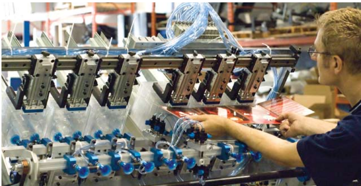
An engineer at Pack-Smart's Toronto factory deftly prepares another rotary pick-and-place machine for pending shipment to a U.S.-based client.
